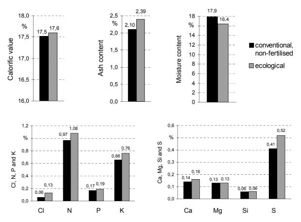
*Figure 23:* Biofuel properties of maize variety Clarica with conventional/non-fertilised and ecological cultivation. All values related to dry basis (d.b.), except moisture (w.b.)
