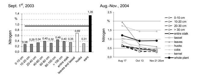
*Figure 15:* Nitrogen content in dry matter of maize plant sections and as a function of time (black line in left graph: whole plant average)
