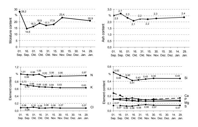
*Figure 10:* Biofuel properties of maize whole plants depending on harvesting time (all data based on dry matter)
