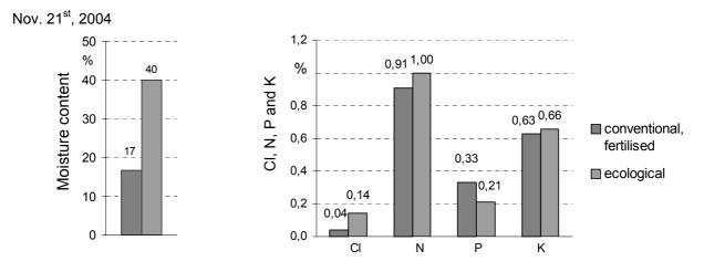
*Figure 24:* Biofuel properties of maize variety Clarica with conventional/fertilised and ecological cultivation. All values related to dry basis (d.b.), except moisture (w.b.)
