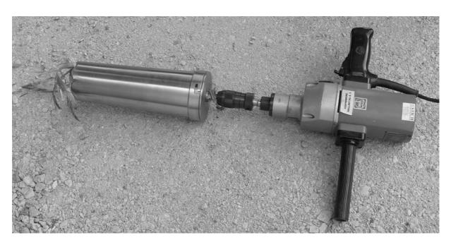
*Figure 8: Core drill for maize bale samplings*
