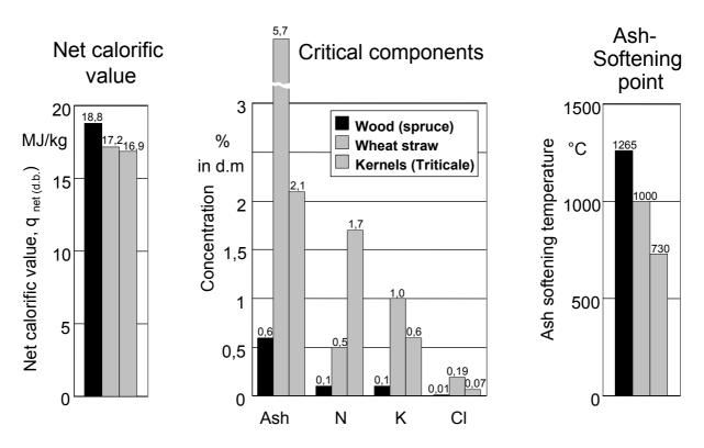
*Figure 9:* Orientation values of biofuel quality characteristics of spruce wood, wheat straw and grain kernels (source: database of TFZ [3])
