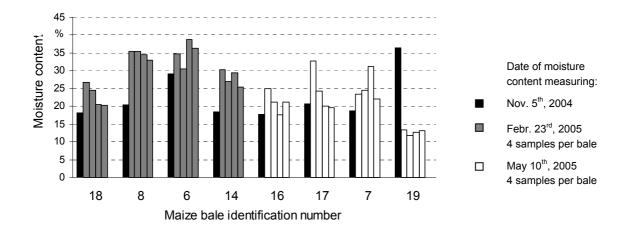
*Figure 28:* Drying intensity of baled maize under plastic covered storage conditions. The average moisture content at storage start was 23 %.
