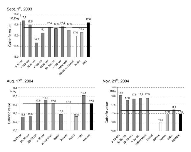
*Figure 12:* Typical calorific values of dry matter of maize plant sections in different years and seasonal stages (black line: whole plant average). All data based on dry matter
