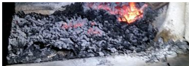
Figure 5: Ash pellets on the grate of a small-scale biomass boiler when firing wheat straw pellets
